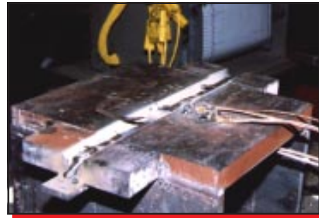
Test plates were restrained for up to 30 days.
