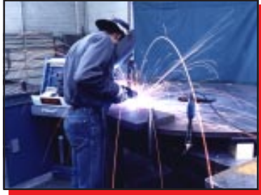
Meta-Lax Weld Conditioning of 6061-T6 test plates.
