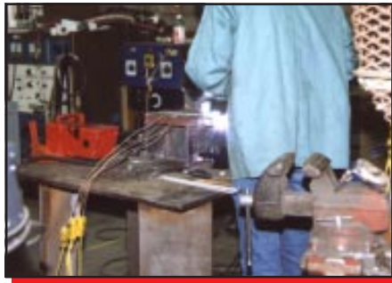
Test plates, A36 (or 4140), being Meta-Lax Weld Conditioned (i.e. Meta-Lax DURING welding).
