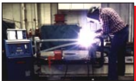
Meta-Lax Weld Conditioning of aluminum fixtures.
